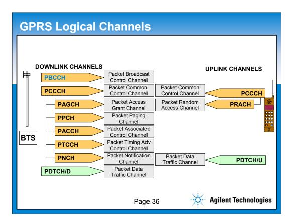
This slide defines each of the logical channels mentioned in the previous slide. The packet data traffic channel (PDTCH) is used to transfer user data
