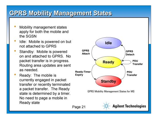
A mobile can be in any of three states depending on its current traffic level. Location update frequency is dependent on the MS state.
