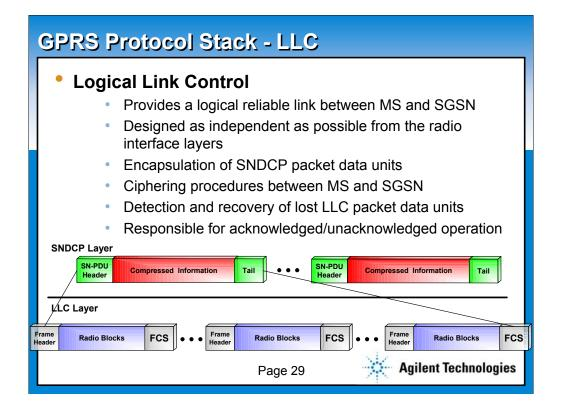
The LLC (Logical Link Control) layer provides the reliable link between MS and SGSN. LLC supports these layer-3 Protocols:
