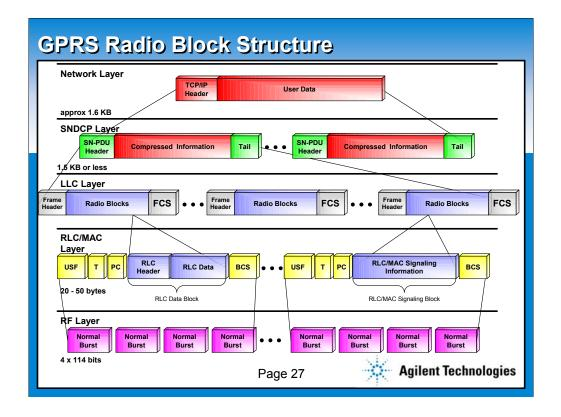
A closer look at the protocol stacks reveals how the data transport occurs. The accompanying diagram illustrates how the headers are attached to the user data as it is transported down each successive layer. This diagram provides an overview of the process. Subsequent slides will provide details on each layer.
