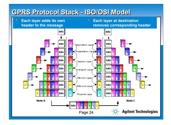
To understand how the protocol stacks provide transmission of data from one layer to the next, refer to the diagram. Let's start with some information ('info') at the top of the Node A stack. To transport that information (text, photo, etc.) over the air interface, the system must add a new header at each successive layer as it travels from top to bottom. For example, at the Application layer, it adds header message #7. By the time it reaches the physical layer, it has added headers 2 through 7.
