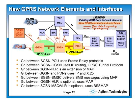
Here's a more detailed look at the GPRS network architecture, including the new network elements and network interfaces.
