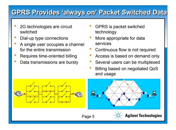
GPRS is a packet-based technology which is optimized for data services. While GSM also provides data services, it is circuit-switched and data speeds are much slower.
