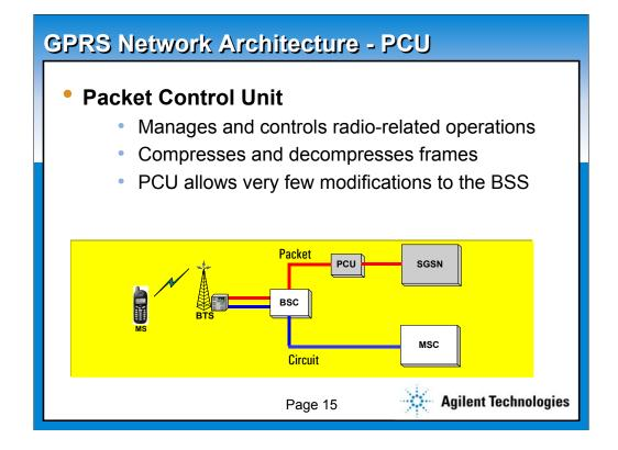
The PCU takes care of the radio resource functionality's like allocation of air interface channel blocks. It will also do packet segmentation due to limitation of bandwidth on the air interface. The PCU will also do some Quality of Service measurements to alter communication parameters on a real time basis.
