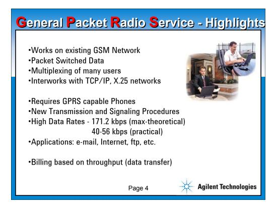
GPRS stands for General Packet Radio Service. We will discuss the key highlights and differences which GPRS brings to the existing GSM network.
