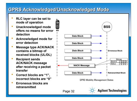
The RLC layer can be set to either Acknowledged or Unacknowledged mode of operation. Unacknowledged mode offers no means of error detection. Acknowledged mode uses error detection. ACK/NACK messages contain a bitmap of received blocks whereby the recipient sends a 1 for correct blocks and a 0 for incorrect blocks. Bad blocks are retransmitted.
