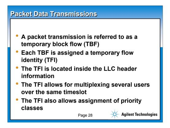
As discussed in the previous slide, a TBF is a physical connection used by the two radio resource (RR) entities to support the unidirectional transfer of Logical Link Control (LLC). A TBF is temporary and is maintained only for the duration of the data transfer. Each TBF is assigned a temporary flow identity (TFI) by the network. The TFI is unique in both directions. It allows for multiplexing several users over the same timeslot, and it can provide the assignment of priority classes.
