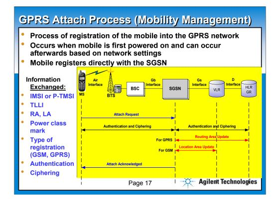
A GPRS Attach is a GMM (GPRS Mobility Management) process. It is always initiated by the mobile. The GPRS default mode does an attach on Power On, and it can also be forced. A GPRS Attach is made to the SGSN.
