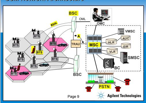
Here is a diagram of a GSM network. The mobile transmits and receives over the air interface. Each base station serves a cell, and handovers occur as the mobile moves from cell to cell. The BTS is connected to the BSC over an Abis link. The BSC connects to the MSC over the A interface. The circuit-switched voice or data calls are then connected to the PSTN.
