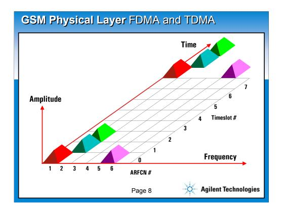
GSM uses TDMA (Time Division Multiple Access) and FDMA (Frequency Division Multiple Access). The slide shows part of one of these bands. Each band is divided into 200 kHz slots called ARFCN's (Absolute Radio Frequency Channel Numbers).
