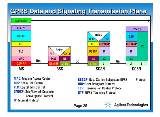
Now, let's specifically look at the GPRS protocol stacks for the mobile, BSS (PCU), SGSN, and GGSN. The physical layer (layer 1) provides the connectivity between the network elements.
