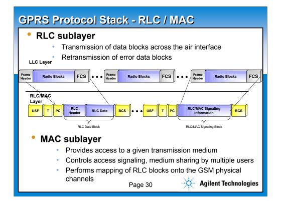
The RLC (Radio Link Control)/MAC (Medium Access Control) layer includes two functions. First, the RLC layer is a reliable link between the MS and BSS. It includes segmentation and reassembly of LLC frames into RLC data blocks.
