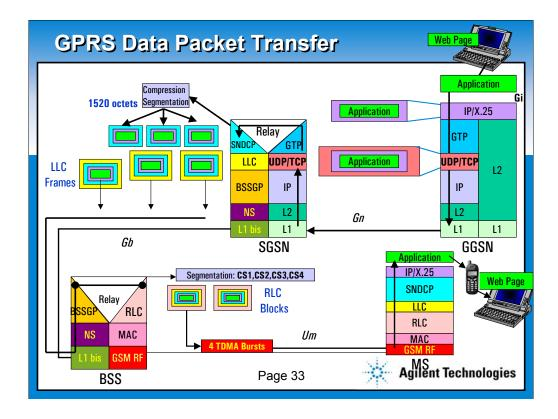
Now that we have a better understanding of the GPRS concepts, let's take an example of how a PDU (packet data unit) is sent from the landline network to a mobile. The user sends a text message from a PC through the Internet to the wireless operator's network and finally to the end user's GPRS wireless data device.
